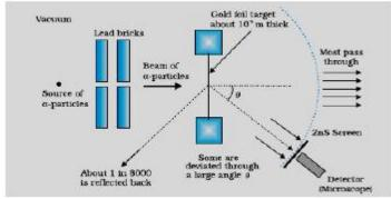
High energetic collimated beam of  $\alpha$ -Particles is allowed to fall on a very thin gold foil as shown. The scattered  $\alpha$ -particles are observed through a rotating detector consisting of ZnS screen and microscope.
