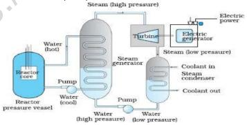
Working: In a nuclear reactor,  $^{235}_{92}U$  is used as a fuel, cadmium rods are used as control rods and graphite or heavy water as moderator. The entire set up is shielded with a heavy thick lead sheets and then with a thick concrete walls. The energy obtained from fission is used to heat up the water to produce steam. This steam is then used to rotate the turbines to produce electricity
