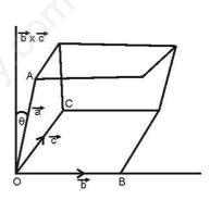
Magnitude of this projection =  $\frac{\vec{a}.(\vec{b} \times \vec{c})}{|\vec{b} \times \vec{c}|}$
