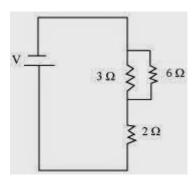
Here, 6  $\Omega$  and 3  $\Omega$  resistors are connected in parallel. Therefore, their equivalent resistance will be given by
